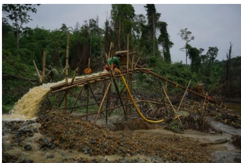
Groundwater is suctioned through a bamboo sluice tray to separate out particles of gold (Yawng Htang | Frontier )
